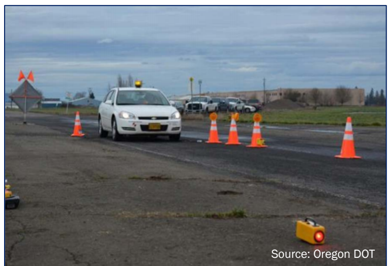
Figure 5: A worker alert system located 50 ft from equipment while activated by an intruding vehicle.
