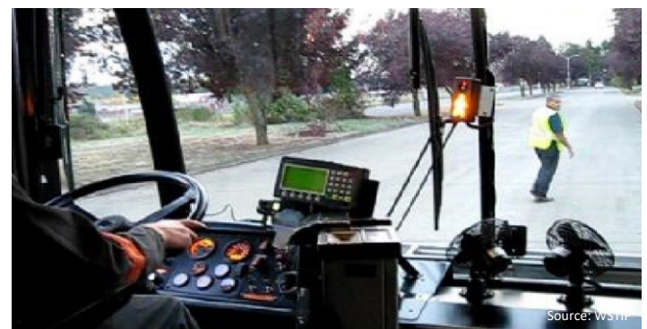
Center indicator illuminates as pedestrian crosses in front of moving bus.
